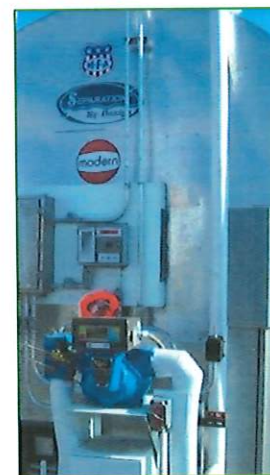
...Series 700 Rotary Meter for biodiesel
