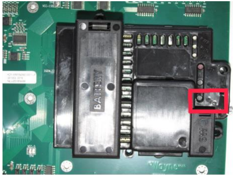
CRC button placement on Wayne iGEM 2 Calculator.
