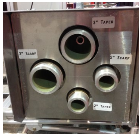
Model 3000 Tool - Tapers and scarfs 2" and 3" Dualoy 3000/LCX pipe.
