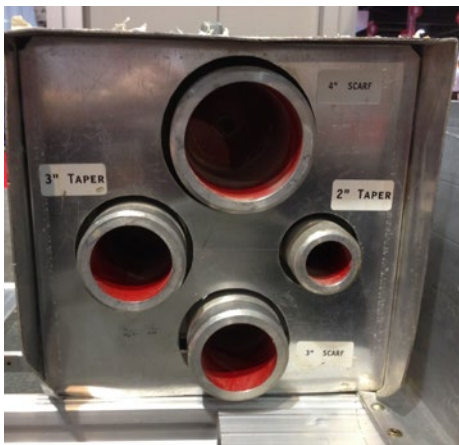
Model 2100 Tool - Tapers 2"-3" Red Thread IIA pipe, scarfs 3"-4" pipe. Taper mandrels are available for Dualoy 3000/L products.
